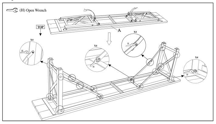
Lay down Bench (A) on padded non-marring surface, lift legs upright to 90 degrees untill the braces are locked, as shown in the diagram. **Tighten 16 nuts on supporting brace using Open Wrench (H). DO NOT OVER TIGHTEN.**
