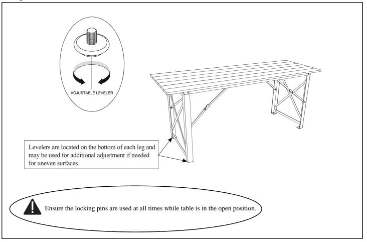
Assembly is now complete and the product is ready for use. Adjustable levelers are located on the bottom of each leg and may be adjusted by turning outwards, counter-clockwise to help account for uneven surfaces. NOTE: Hardware may loosen over time. Periodically check that all connections remain tight and adjust as needed.
