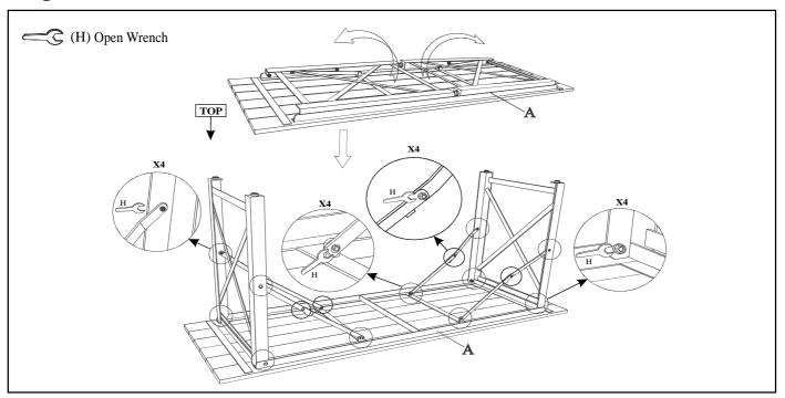
Lay down Table (A) on padded non-marring surface, lift legs upright to 90 degrees untill the braces are locked, as shown in the diagram. **Tighten 16 nuts on supporting brace using Open Wrench (H). DO NOT OVER TIGHTEN.**
